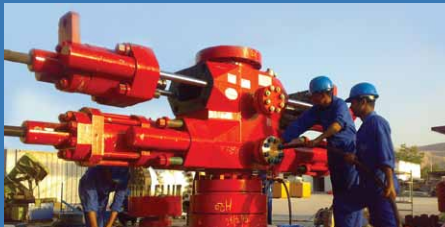
MAINTENANCE OF BOP
