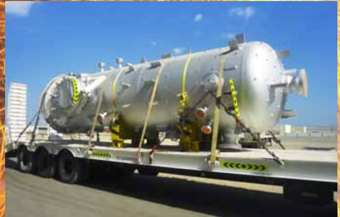
INCONEL 625 CLADDED TEST SEPARATORS
