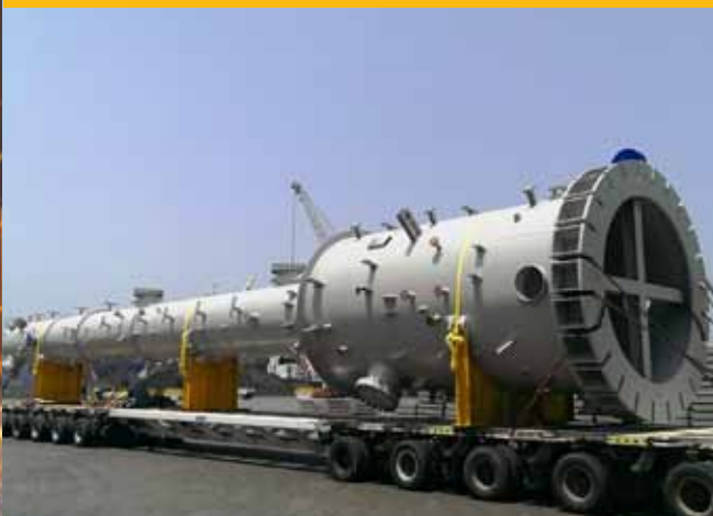
SOUR WATER STRIPPER COLUMN
